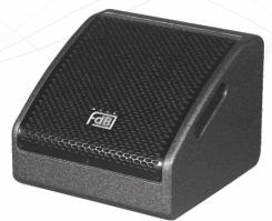
MR108C is a compact, small size, coaxial 2-way full range monitor speaker. It uses 1x8" high efficency mid-bass unit and 1x1" exit throat 44mm voice coil HF driver with horn. The wood box adopts multilayer composite plywood, wear-resistant and waterproof polyurea paint. MR108CA is equipped with FA1.3 digital amplifier module based on MR108C to be an active speaker.
