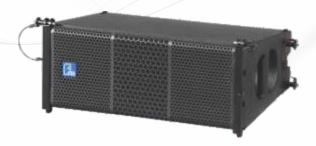
The MLA206 is a mini line array loudspeaker for small and medium scale sound reinforcement, fitted with two 6" LF neodymium drivers and one 1" neodymium HF driver coupled to a patent line array horn, made of high quality plywood with polyurea waterproof paint. All rigging parts are made of aluminium alloy.
