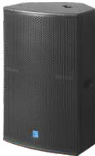
The LH15H is the ideal general-purpose 2-way loudspeaker with a wide frequency response, suitable for all kinds of mid-field theatre and live venue applications that require professional sound quality, fitted with one 15" neodymium woofer and one 1.4" exit neodymium compression driver coupled to a rotatable horn.
