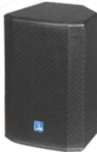
**S110 is a 10" 2-way full range speaker.** It uses 1x10" high efficiency mid-bass unit, 1x1"exit throat 44mm voice coil HF driver with 90°×50° rotatable horn.The wood box adopts multilayer composite plywood with special environmental protection paint.
