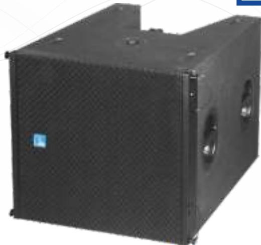
**DLA118B is a single 18" subwoofer.** It uses 1x18" 100mm voice coil woofer,bass-reflex design,hanging system adopts aluminum alloy material, can be hung, supported,stacked with DLA208 and DLA112. The wood box adopts multilayer composite plywood, wear-resistant and waterproof polyurea paint. DLA118BAS is equipped with SA2.68 digital amplifier module based on DLA118B to be an active system with DLA208 and DLA112.
