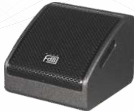
MR108C is a compact, small size, coaxial 2-way full range monitor speaker. It uses 1x8" high efficiency mid-bass unit and 1x1" exit throat 44mm voice coil HF driver with horn. The wood box adopts multilayer composite plywood, wear-resistant and waterproof polyurea paint. MR108CA is equipped with FA1.3 digital amplifier module based on MR108C to be an active speaker.
