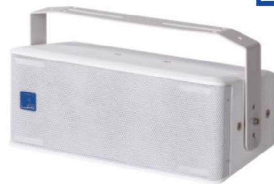
The MINI 205 is a two-way loudspeaker system with two 5" woofer and 1" exit compression driver coupled to a round 140°×140° wide dispersion horn.
