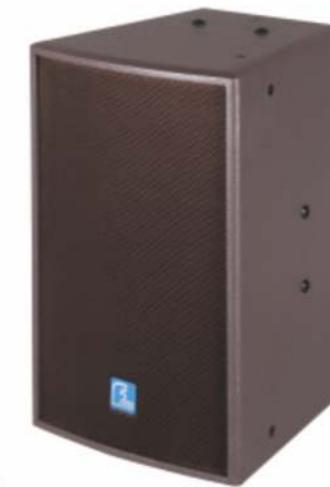
The KH10 is a two-way full-range loudspeaker designed for KTV rooms, made of high quality plywood, back vented design. Fitted with one 10" woofer and one 1" exit compression driver coupled to a rotatable horn.
