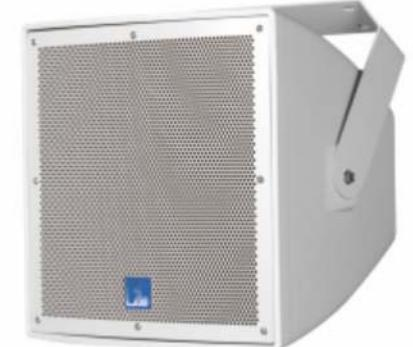
The LT208 is a compact, 8" coaxial-driver, 2-way, highly weather-resistant, full range loudspeaker with high SPL, the body is made of engineering plastic injection molding. The system conforms to IP56 international standard. LT208T is equipped with multi-tap transformer based on LT208.
