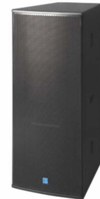
The LH215 is the ideal general-purpose 2-way loudspeaker with a wide frequency response, suitable for all kinds of mid-field theatre and live venue applications that require professional sound quality, fitted with two 15" neodymium woofers and one 2" exit neodymium compression driver coupled to a special design horn.
