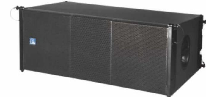
The **MLA212** is a 2.5-way line array loudspeaker for long throw distance scale sound reinforcement, fitted with two 12" neodymium LF driver and two 1.4" neodymium HF driver, made of high quality plywood with polyurea waterproof paint. All rigging parts are made of aluminium alloy. The **MLA212DA** is equipped with FA2.38 digital amplifier module based on **MLA212** to be an active line array loudspeaker.
