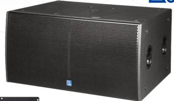
MLA221B is a dual 21" low frequency enclosure designed for sub-bass reinforcement to MLA series, made of high quality plywood with polyurea waterproof paint, fitted with two 21" woofer with 4.5" high temperature voice coil. MLA221BA is equipped with BA2.13 digital amplifier module based on MLA121B to be an active subwoofer.
