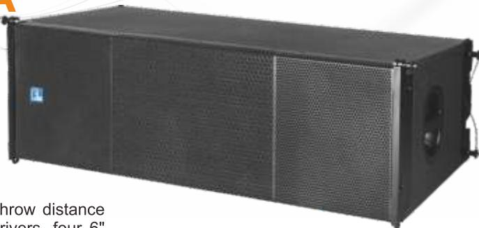
The MLA8312 is a 3-way line array loudspeaker for long throw distance sound reinforcement, fitted with two 12" neodymium LF drivers, four 6" neodymium MID drivers and two 1.4" neodymium HF driver coupled to 1"x 6" line array horn, made of high quality plywood with polyurea waterproof paint. All rigging parts are made of aluminium alloy. MLA8312DA is equipped with FA2.38 digital amplifier module based on MLA8312 to be an active line array loudspeaker.
