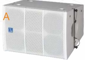
The MLA406 is a mini line array loudspeaker for small and medium scale sound reinforcement. MLA406 is a 2.5-way design housing fitted with four 6" neodymium LF drivers and two 1" neodymium HF drivers coupled to a patent line array horn, made of high quality plywood with special environmental protection paint. MLA406A is equipped FA1.6 digital amplifier module to be active loudspeaker based on MLA406.
