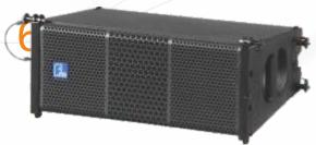
The MLA206 is a mini line array loudspeaker for small and medium scale sound reinforcement, fitted with two 6" LF neodymium drivers and one 1" neodymium HF driver coupled to a patent line array horn, made of high quality plywood with polyurea waterproof paint. All rigging parts are made of aluminium alloy.
